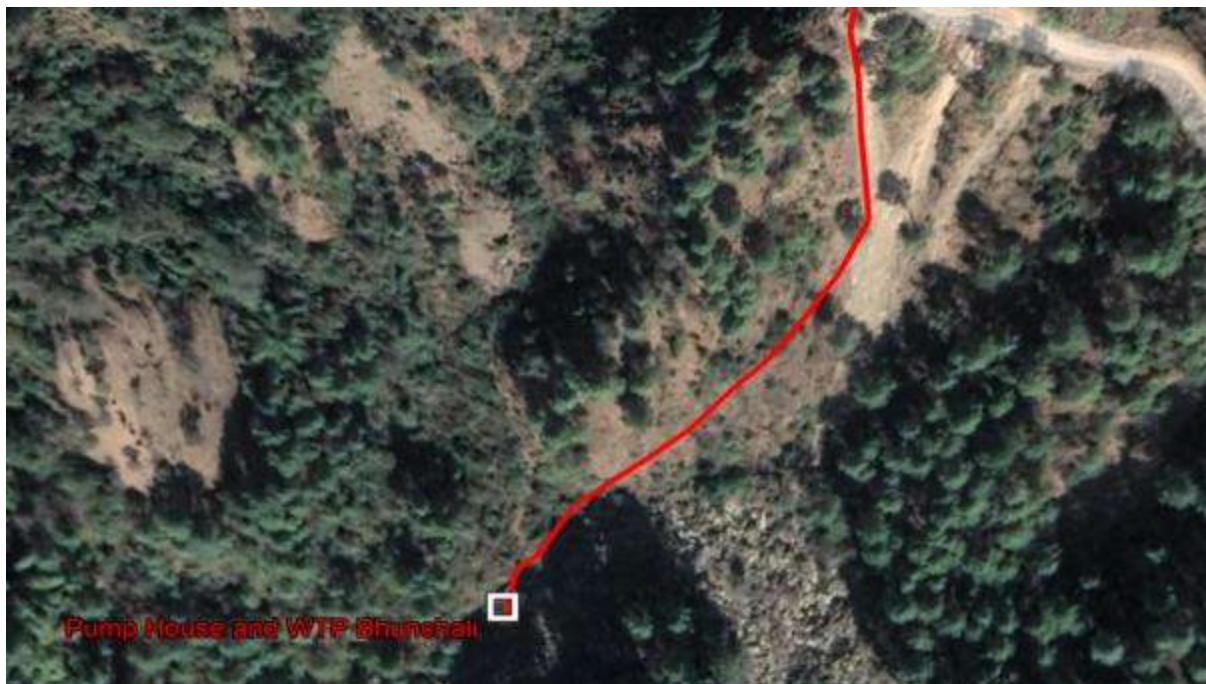
Grid MS-2: Alignment of Rising main from PH through Kaccha path to Main Road.
