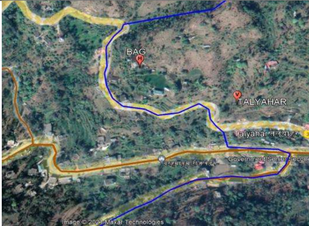
MS-2: Proposed distribution Network on State Highway 26
