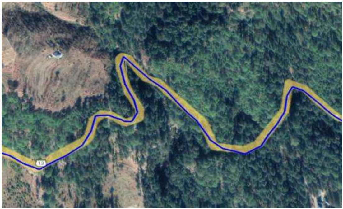
MS-15: Proposed Gravity Main on State Highway 13 near SR Juanga (80-150mm)
