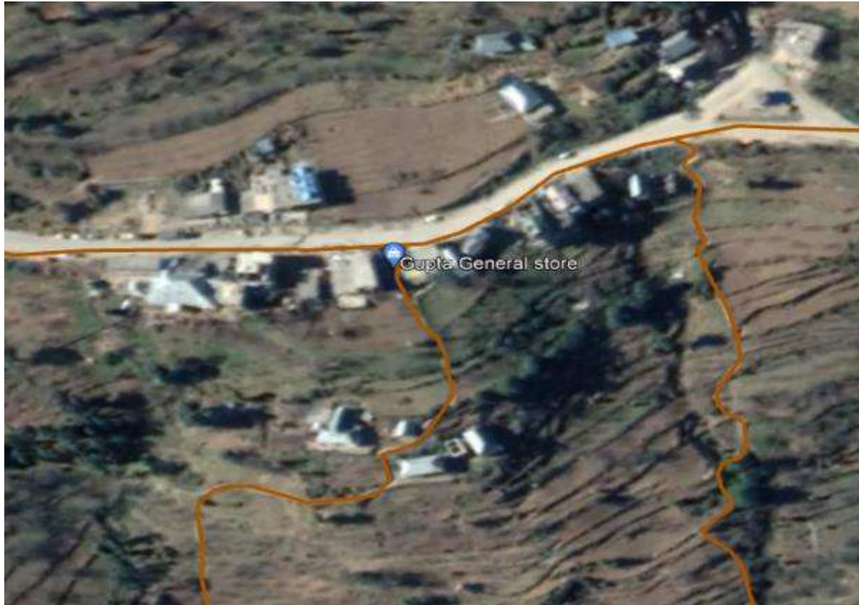
Grid MS 6: Alignment of Gravity Main from Source along with forest trails/ water stream
