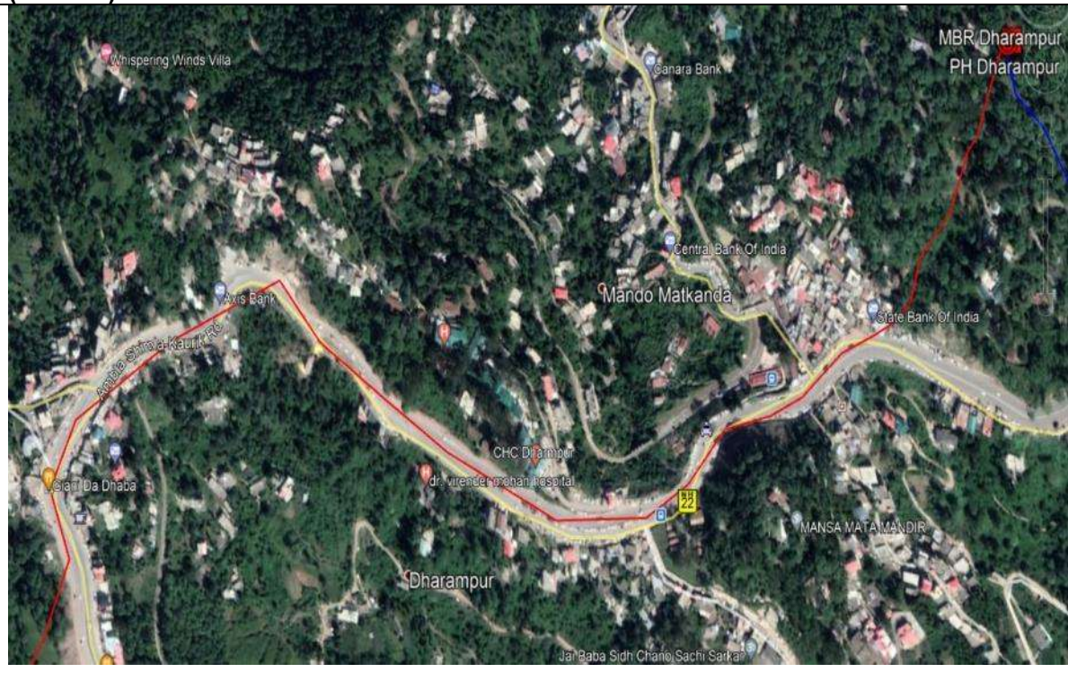
SS1: Prop Rising Main from PH Dharampur to MBR Kasauli on National Highway 22 (200mm)
