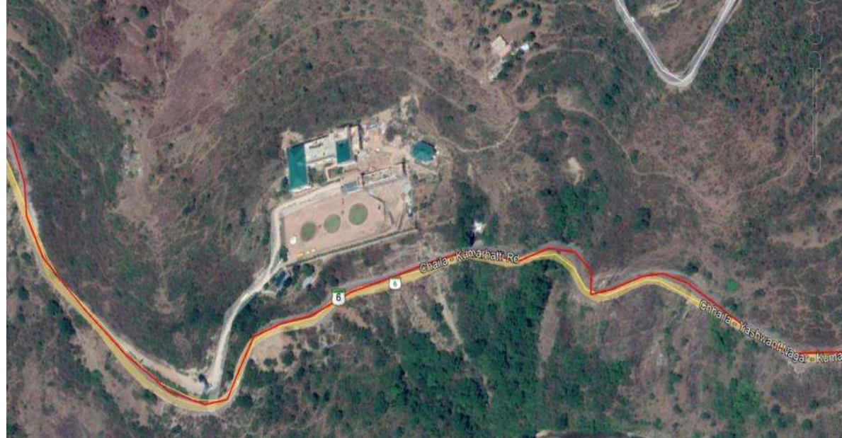
SS1: Proposed Rising Main on State Highway 6 from Pump house near Proposed WTP at Giri River to Proposed Sumpwell Stage-2 Bigad, (200 mm)
