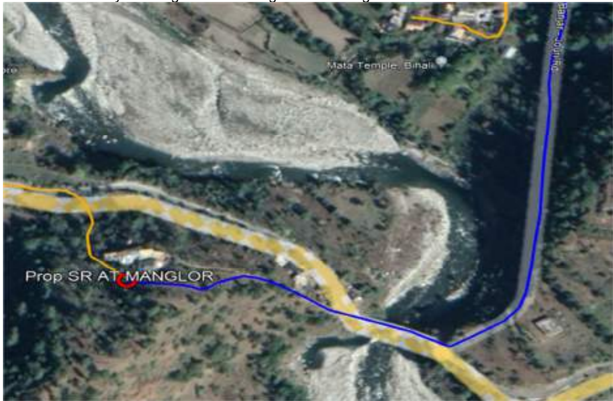
Grid MK 6: Alignment of Gravity Main from SR along village roads.
