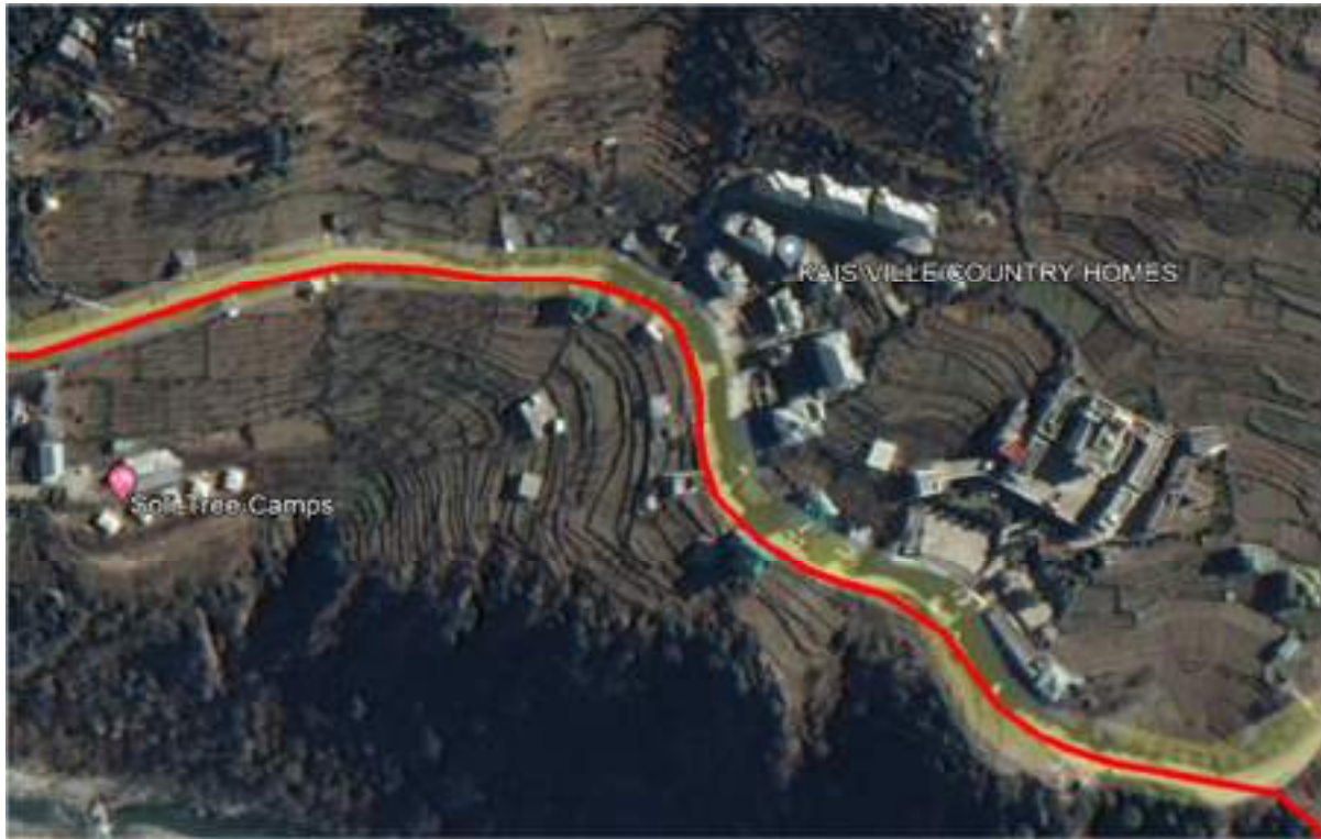
MK 9: Proposed alignment of Gravity Main along NH 305 (150-200mm)
